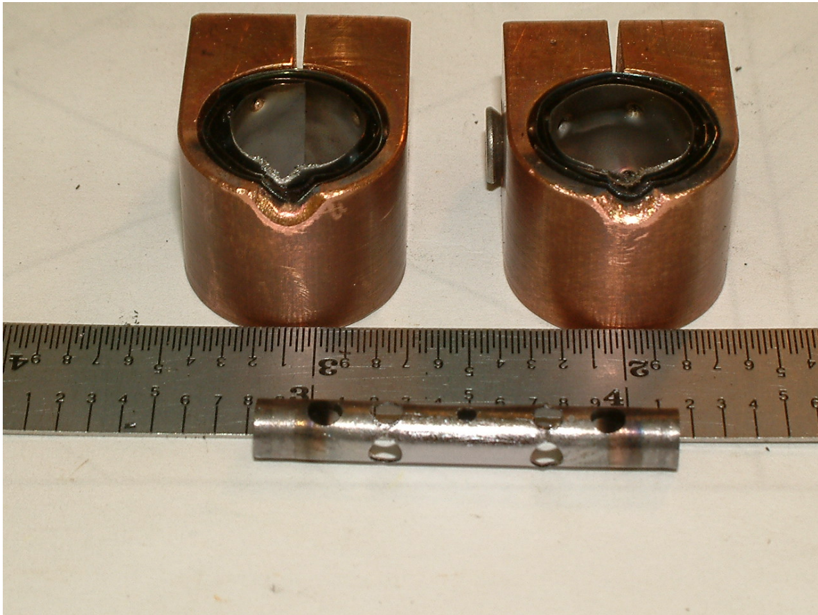
FIG. 2. The copper clamps and the detached, tantalum crucible.
